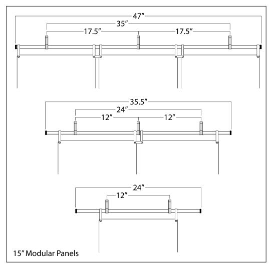
1. **Tape Template and Drill.** Tape the provided template to the ceiling or wall where Modular Panels will be placed. Drill the needed holes using the holes in the template. Use a 1/8" drill bit when using just screws, and a 3/16" drill bit for the drywall anchers.
