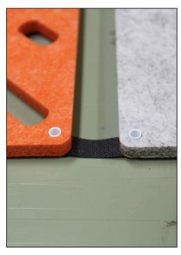
3. Insert the screw side of the barrel into another fabric connector. Place the screw side of the barrel into the open end barrel from the previous step. Don't press the barrel all the way together yet. Be sure not to pinch the fabric connector in between the halves of the barrel. If this happens pull the two halves apart with pliers or two screwdrivers. More pictures of the process is on the following page.
