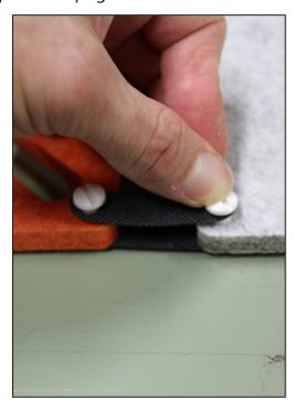
4. Using a hard flat object, push the barrels together. Leave a small gap between the two halve so the fabric connectors have the ability to move.
